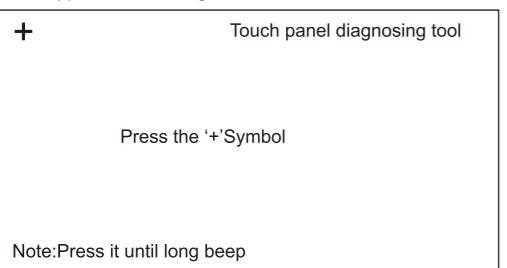
Click top left corner, top right corner, bottom right corner , bottom left corner and the center of '+' in turn and restart.
